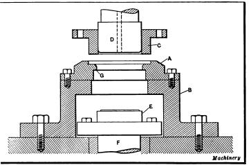
Fig. 10. Triple-action Die for Blanking, Drawing, and Embossing
